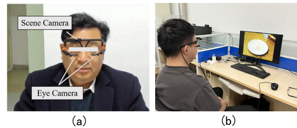
Fig. 1. The wearing standard illustration (a) and experimental real scene (b) of Pupil Core.
